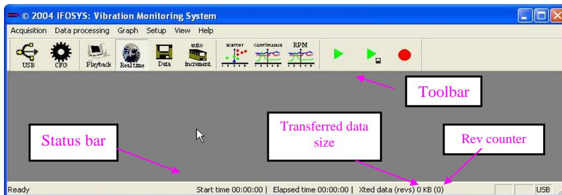
window shows the start time, elapsed time, size of data transmitted to the buffer (or file), revolution counter, and three system state boxes, which indicate state of the system, that is, **USB** connected, **ACQ** – acquiring data and **REC** – saving to file. The left area of the main window can be used to view current workspace, which shows all the files.
