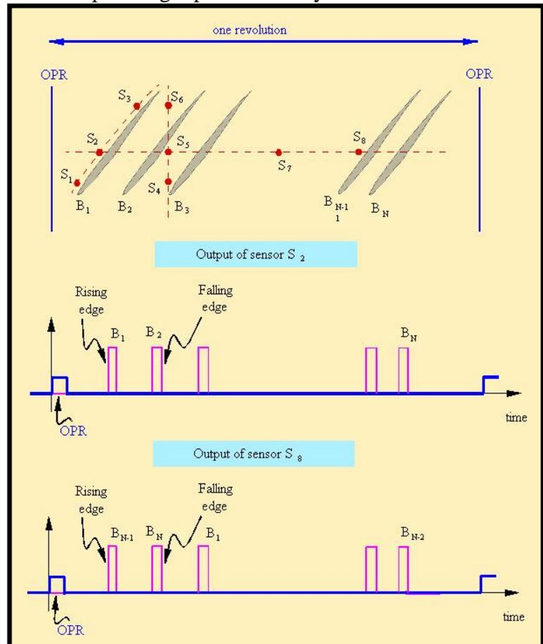
example, along the circumference of the engine casing, that is, S2, S5, S7 and S8; or parallel to the axis of the rotor, that is, S4, S5 and S6; or parallel to the blade chord, that is, S1, S2 and S3. Each sensor produces a sequence of pulses representing each blade tip. The VMS2000 timing board measures time location of each blade edge, referenced to the once-per-revolution (OPR) signal. Each time event is measured using a 50 MHz oscillator and is represented by a 24 bit count vector,
